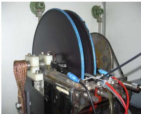
Fig. 7.a. Black powder direct after test start
