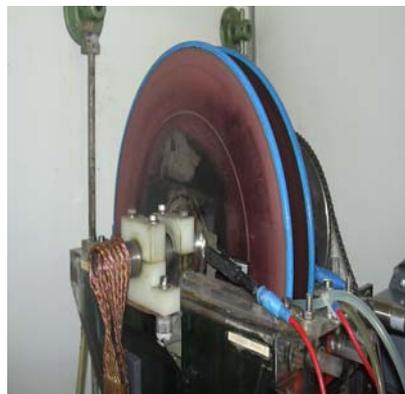
Fig. 7.b. A dark reddish gray deposition after 60 min
