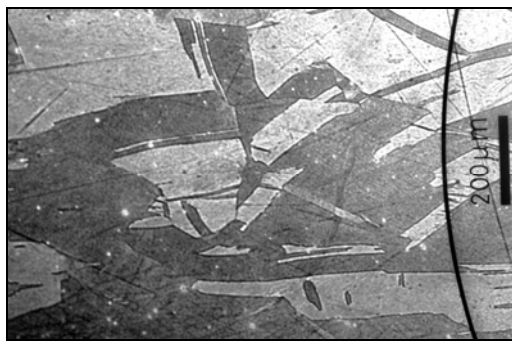
Figure 4: Microstructure of cold deformed Cu strip
