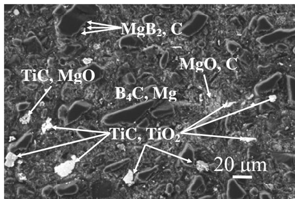
Fig.4. SEM-EDS of composite sample 6 (Table 1)
