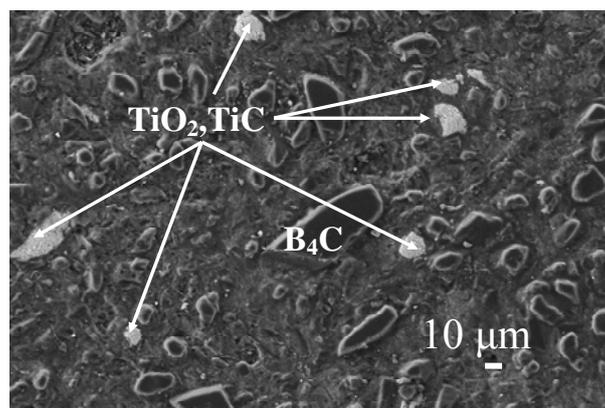
Fig.5. SEM-EDS of composite sample 7 (Table 1)
