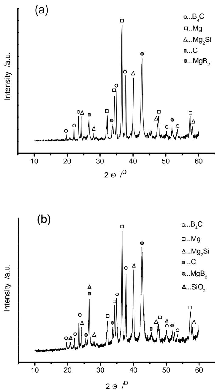
Fig.6 a, b. XRD of composite samples: (a) sample 4 (Table 1)-wetting agent Si, (b) sample 8 (Table 1)-wetting agent Ti
