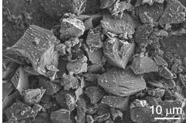
*Fig.1. SEM photograph of B<sub>4</sub>C powder A*
