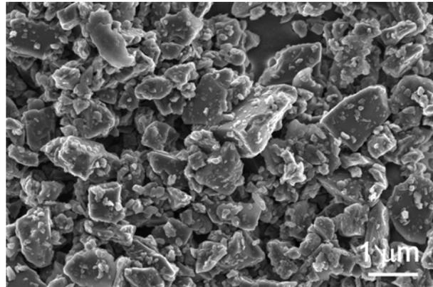
*Fig.2. SEM photograph of B<sub>4</sub>C powder B*
