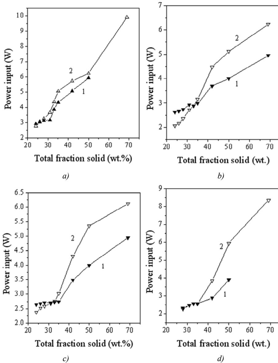
Figure 3. Mixing power dependence on total solid fraction during SSMs mixing: 1) According to the theoretical expression [14]; 2) Electric method. a) ZA27 alloy, b) ZA27 + 3 wt. % Al<sub>2</sub>O<sub>3</sub>, c) ZA27 + 8 wt. % Al<sub>2</sub>O<sub>3</sub>, d) ZA27 + 16 wt. % Al<sub>2</sub>O<sub>3</sub>.
