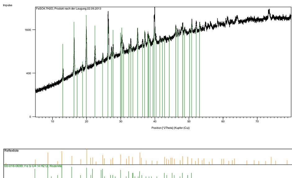
Fig. 11. X-ray diffraction pattern of the produced copperas
