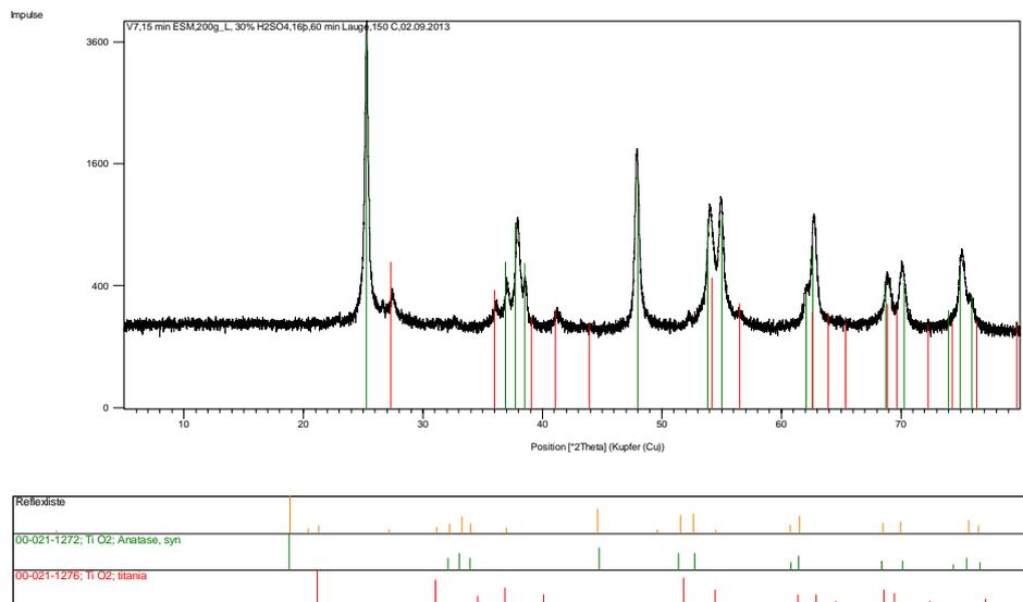
Fig. 10. X-ray diffraction pattern of the produced synthetic anatase
