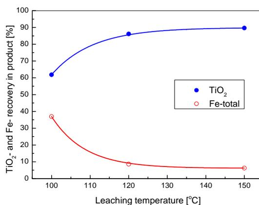
*Fig. 4. Influence of the leaching temperature on the precipitation of anatase upon increasing the amount of reduction agent from 6 to 10% Fe-powder; solids content 50 g/L, 15 min eccentric vibratory milling, leaching time 60 min, 30% H<sub>2</sub>SO<sub>4</sub>*
