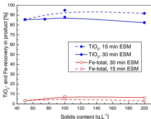
Fig. 8. Influence of the solids content on the precipitation of anatase; leaching temperature 150°C, 15/30 min eccentric vibratory milling, 30% H<sub>2</sub>SO<sub>4</sub>, 6% Fe-powder
