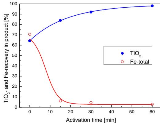
Fig. 2. Influence of the activation time of ilmenite on the precipitation of anatase; leaching temperature 150°C, solids content 50 g/l, leaching time 60 min, 30% H<sub>2</sub>SO<sub>4</sub>, 12% Fe-powder
