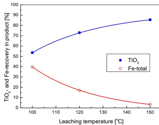
Fig. 3. Influence of the leaching temperature on the precipitation of anatase; solids content 50 g/l, 15 min eccentric vibratory milling, leaching time 60 min, 30% H<sub>2</sub>SO<sub>4</sub>, 6% Fe-powder
